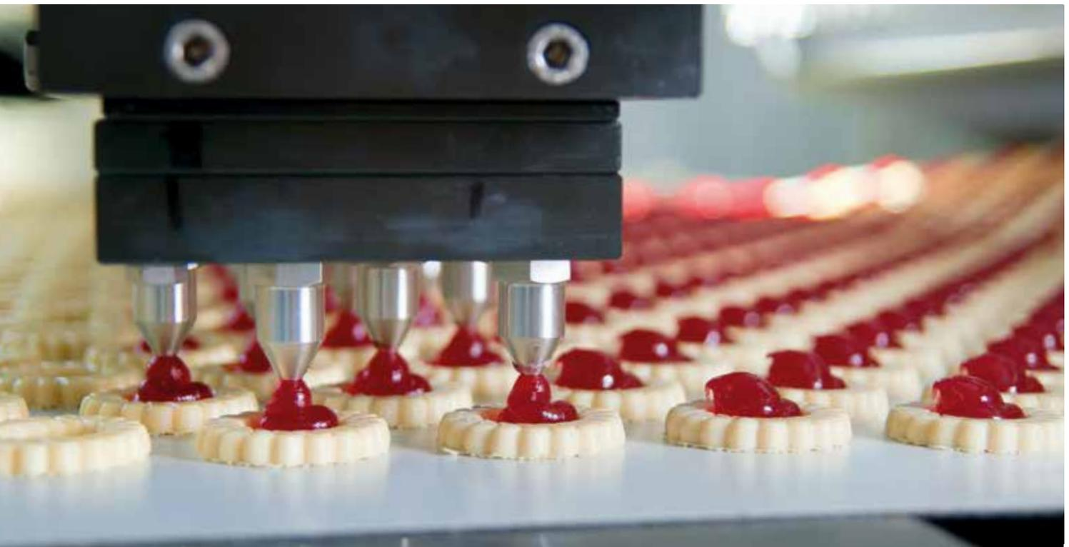
**Portioning units** require high to extremely high corrosion resistance, depending on the foodstuff, and therefore require certification for acidic foodstuffs (pH < 4.5) or testing for aqueous foodstuffs (pH > 4.5).
