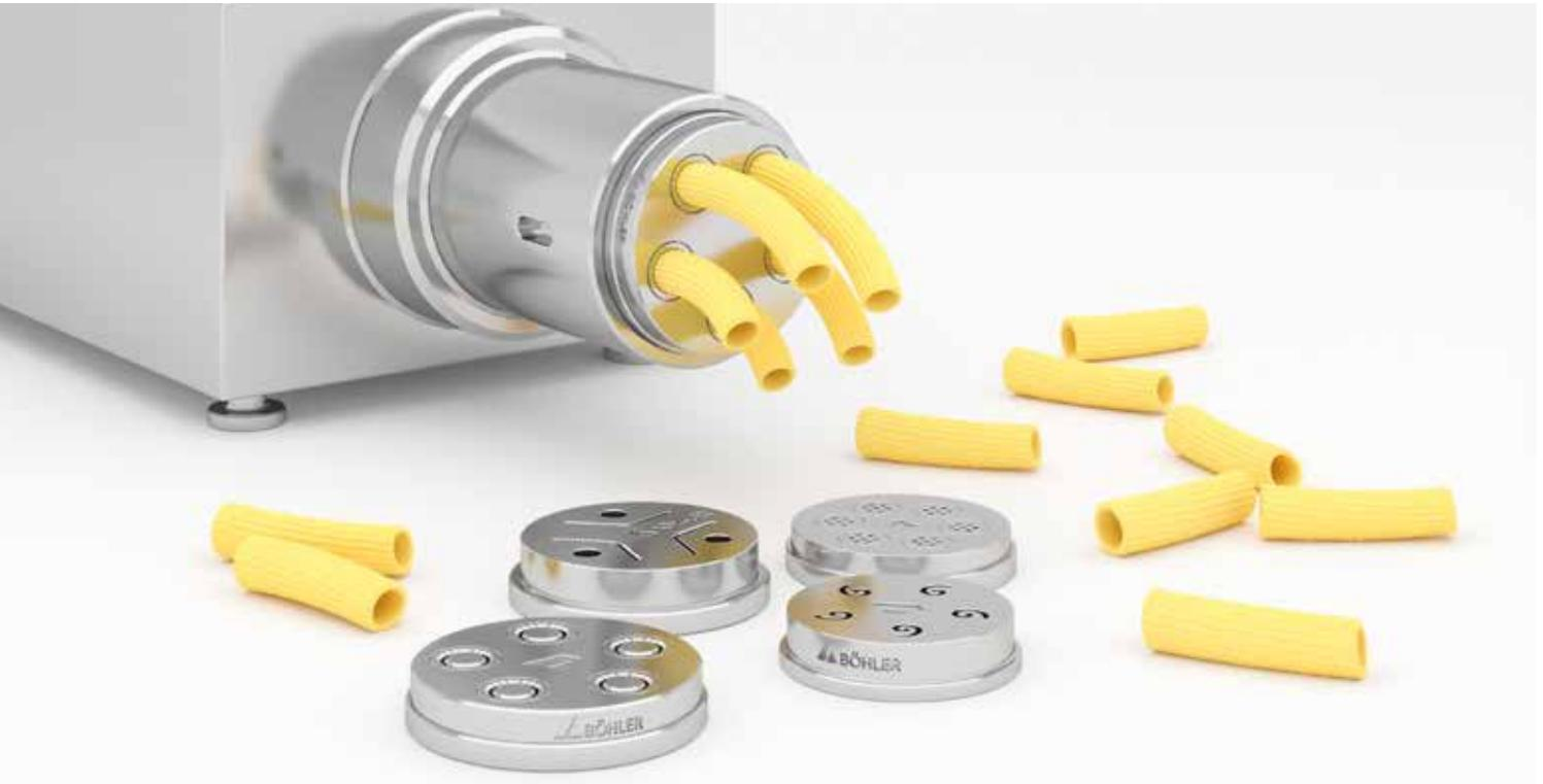
**Extrusion** is industrially used in the production of many foods. Extruders knead, mix, cook and portion foods. This leads to high demands with regard to force and wear, which can only be economically met by tool steels with extremely high resistance to pressure and wear.
