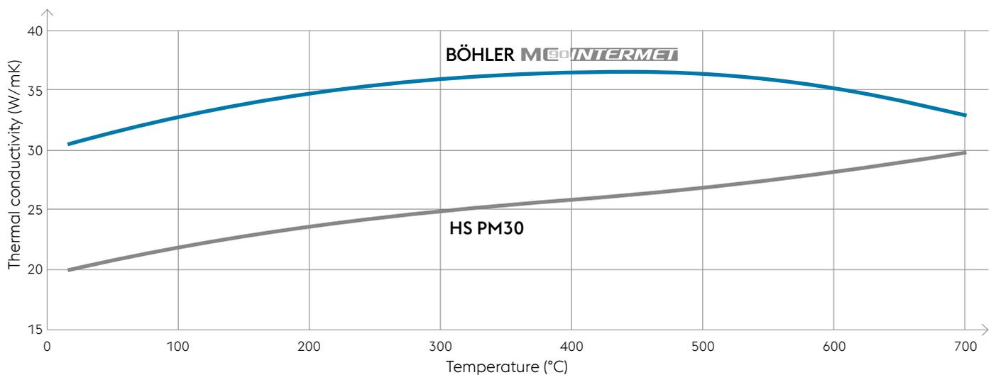
The new cutting material's very high thermal conductivity reduces any effective thermal loading in operation.
