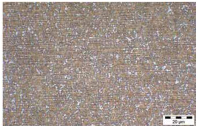
Primary carbides (white) which are embedded in a tempered high speed steel matrix.
