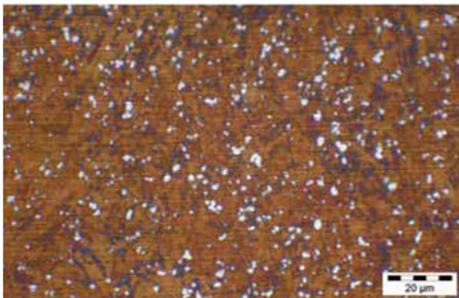
Intermetallic phases (white) which are embedded in a precipitation hardened matrix.
